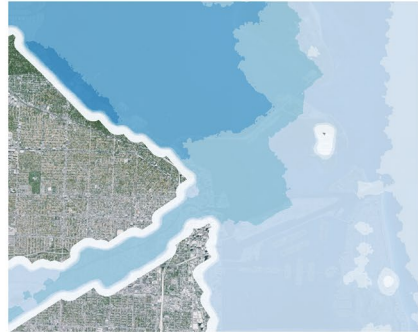
Panel 4. Difference between Category 1 water level map and elevation, used to identify inundation
