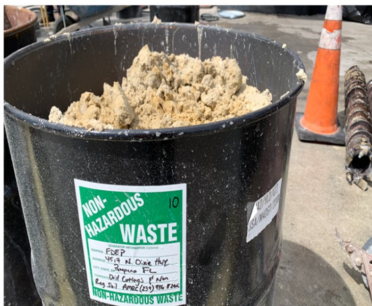
Figure 1. An example of acceptable photo documentation of a drum of soil is provided above. The drum is at least 75% full of soil and numbered to identify the drum from others in the disposal.
