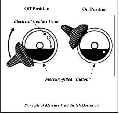
operation and very long operating lifetimes. The mercury-containing buttons can not be broken without the application of excessive force.
