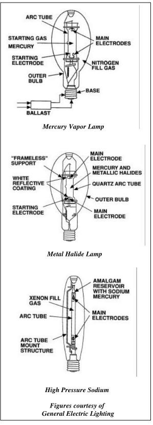
metal halide lamps have very good efficiency, long life, and superior optical control but
