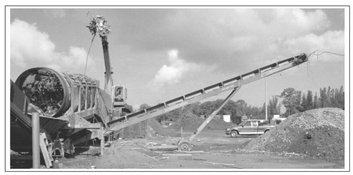
**Recovered Fines Being Produced at a C&D Waste Recycling Facility**
